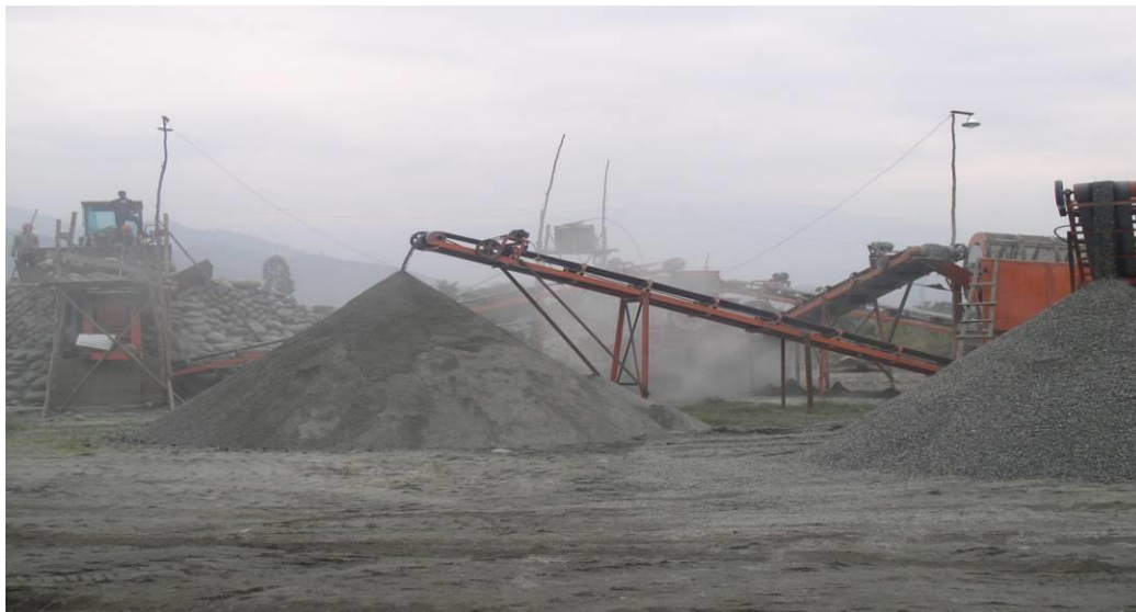
Plate 2.3: Crushing stones that were originally removed from the Mubuku river
